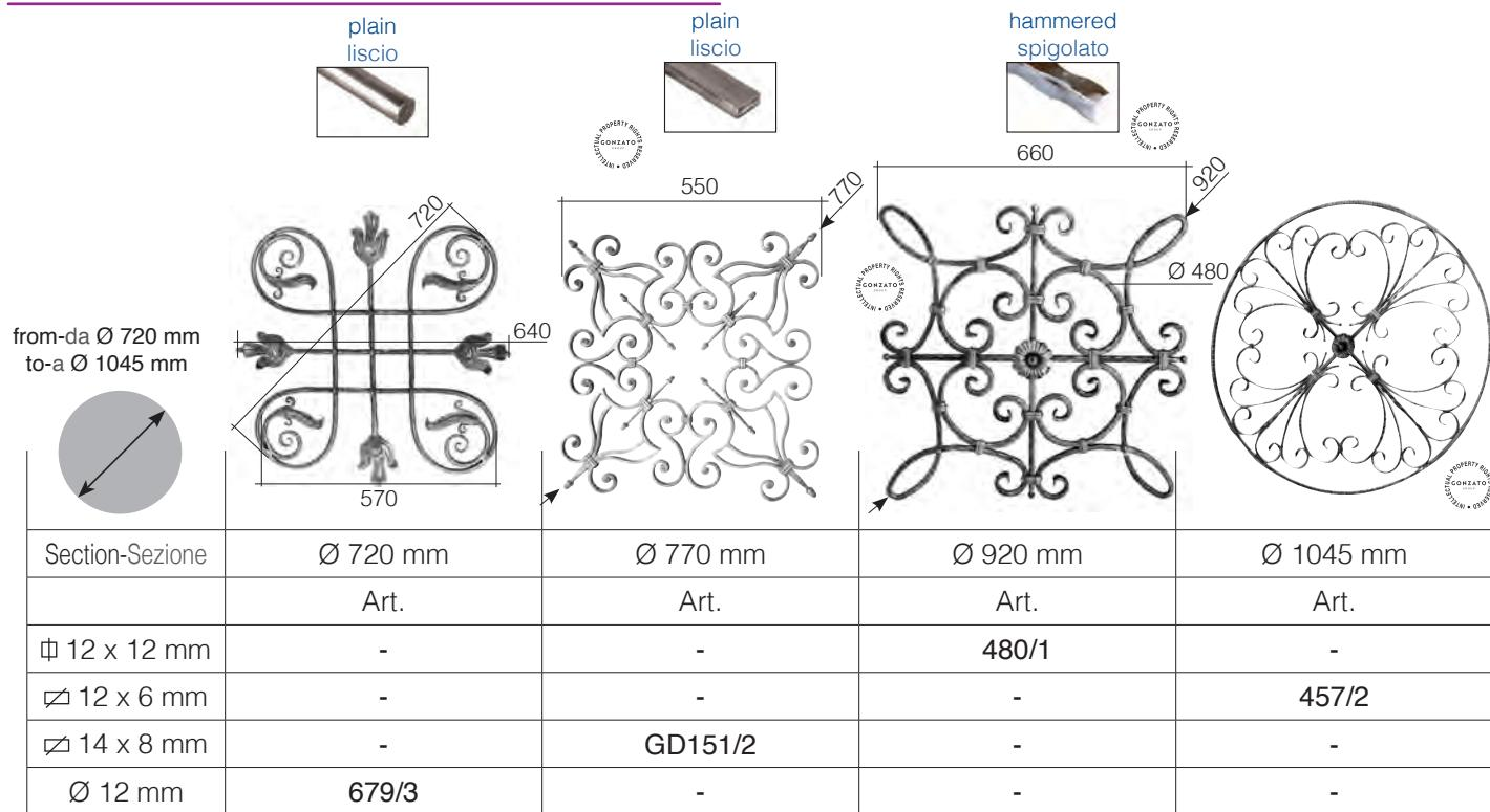
The technical drawing illustrates four different wrought-iron rosette designs, each with specific dimensions and material options:
