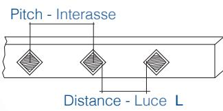
**The punched plates can also be made to measure up to 6 metres.**
