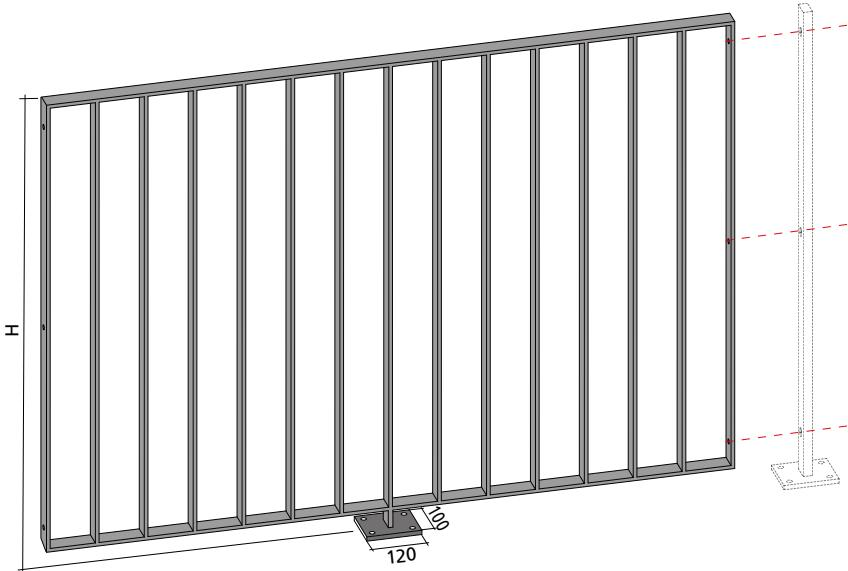
Perimeter structure and infill with vertical plates 40 x 8 mm
