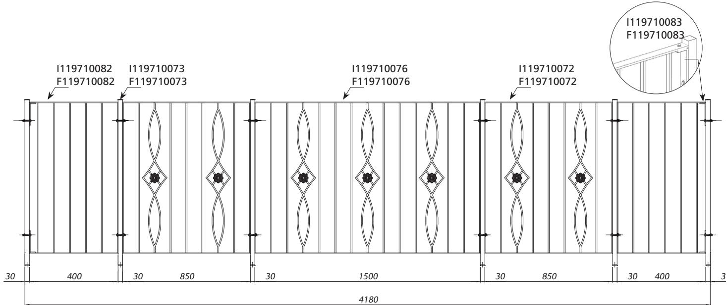
DIRECT ASSEMBLY OF THE PANEL WITH THE NEWEL POST - MONTAGE DIRECT DU PANNEAU AVEC LE MONTANT
