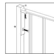
Fasten the angle bracket with screws to the panel and newel post
