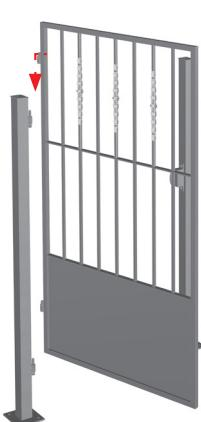
**4** Continue the newel post/standard panel assembly along the required length. To complete the fence exactly to the required size, use a compensating panel if necessary, following the diagram below.
