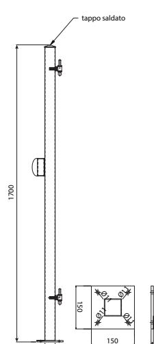
Floor anchoring using mechanical or chemical anchors
