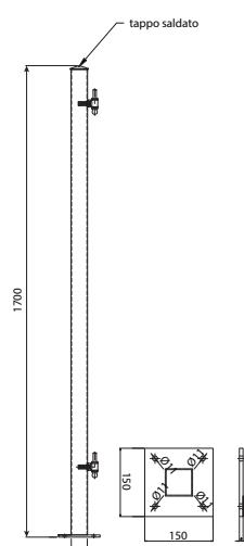
Floor anchoring using mechanical or chemical anchors
