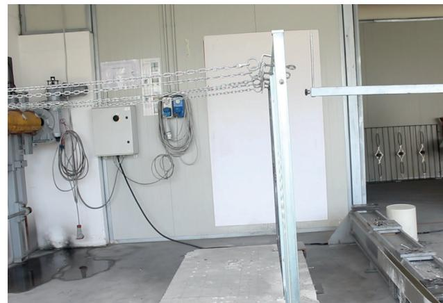
Following the test, the product complied with a strength of **1.5kN/m** with deformations < 100mm
