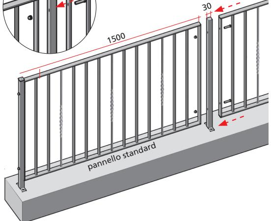
**1** Fasten the first post using the most suitable dowels for the positioning surface.
